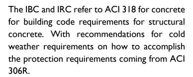
ACI 318 Section 5.12 states that adequate equipment shall be provided for heating concrete materials and protecting concrete during freezing or near-freezing weather. That all concrete shall not come in contact with materials covered in frost and that frozen materials or those containing ice should not be used.
